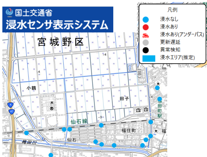
MLIT Flood Sensor System
